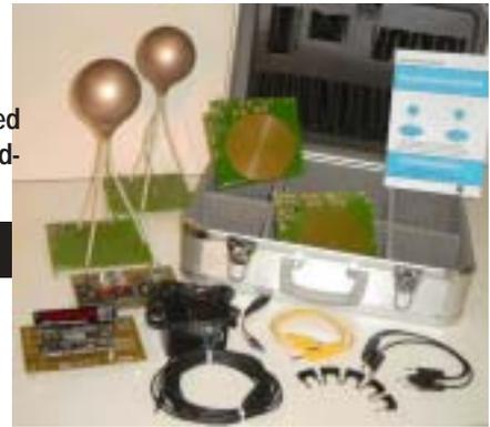
operable beyond the close range. The energy is transferred with the same carrier wave as the information and not over two separated ways as with RFID systems. Besides the bi-directional signal transmission, the energy transfer in both directions is additionally possible because of the resonant coupling between transmitter and receiver.
