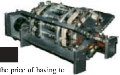
at the price of having to spin a heavy armature. Interference disc generators are more efficient than standard generators because the only moving parts are the “interference” disks which are much lighter than armatures, however, they cannot be used as motors. If current is fed to the coils, the energy is wasted as heat and the disks do not rotate.
