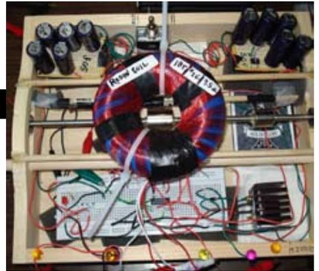
A secondary function of the motor is the charging function provided by the collapsing magnetic fields which occur during each motor pulse. These voltage spikes are fed to a diode and on to the charging item, which may include batteries and capacitors. A portion of the input energy to the motor is recaptured in this manner. The motor is setup to run solely on Supercapacitors as an option, to see how well the charge function recaptures the incident source energy.
